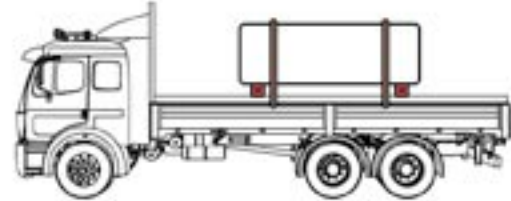
Acceptable securement of a cubic shaped boulder
