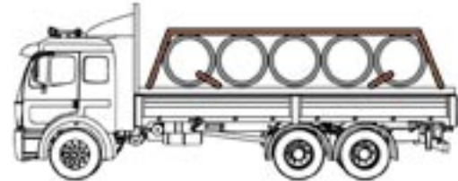
Appropriate stabilization of bottom tier
