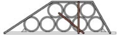
Correct securement of front pipe in partial
