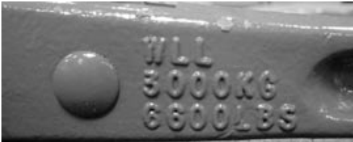
Indicator of Working Load Limit
