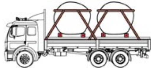
Acceptable securement of a non-cubic Shaped boulder with an unstable base
