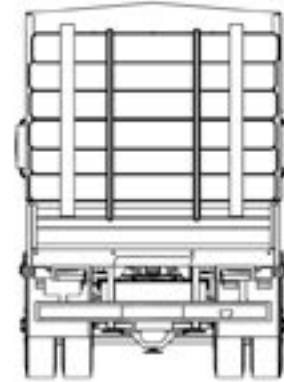
Acceptable securement of one stack loaded crosswise
