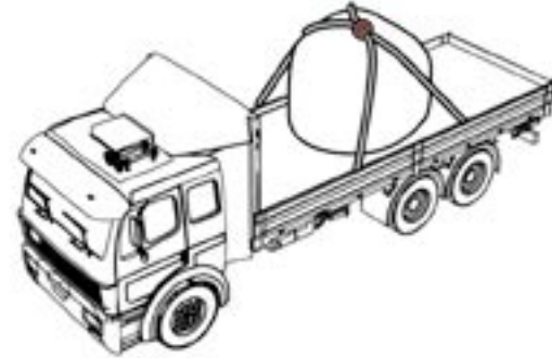
Acceptable securement of a non-cubic Shaped boulder with a stable base
