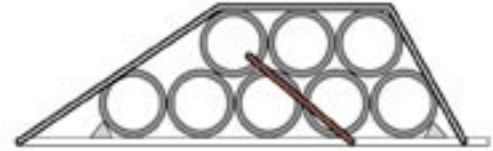
Correct securement of front pipe in partial second tier
