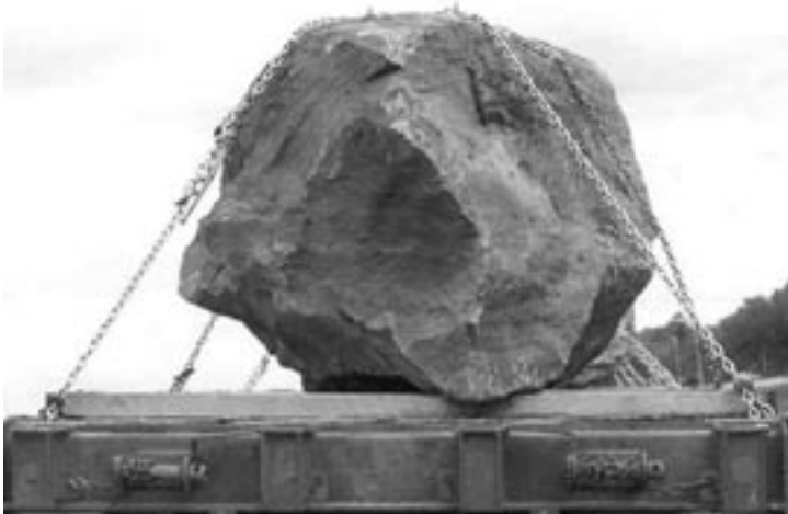
Chain is used to secure large boulders
