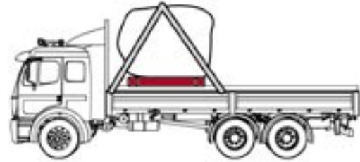
Hardwood blocking pieces placed under the boulder
