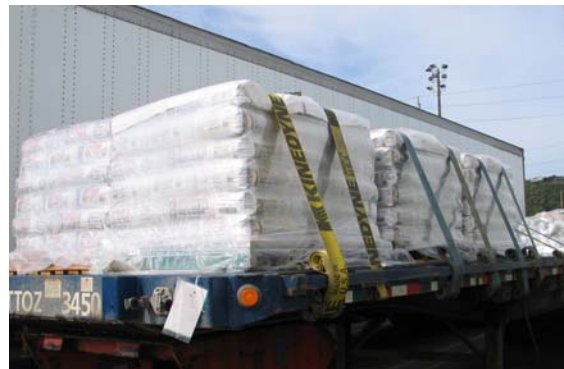
An example of straps cutting into bags as wood softeners were not used.
