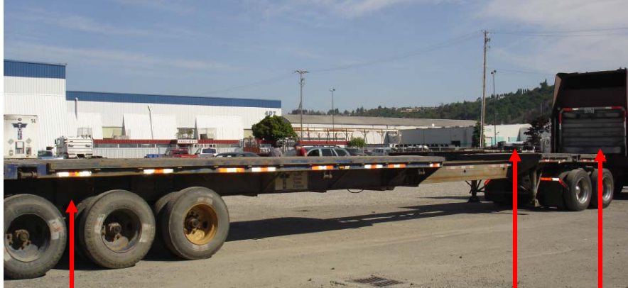
Support load over suspension and king pin areas
